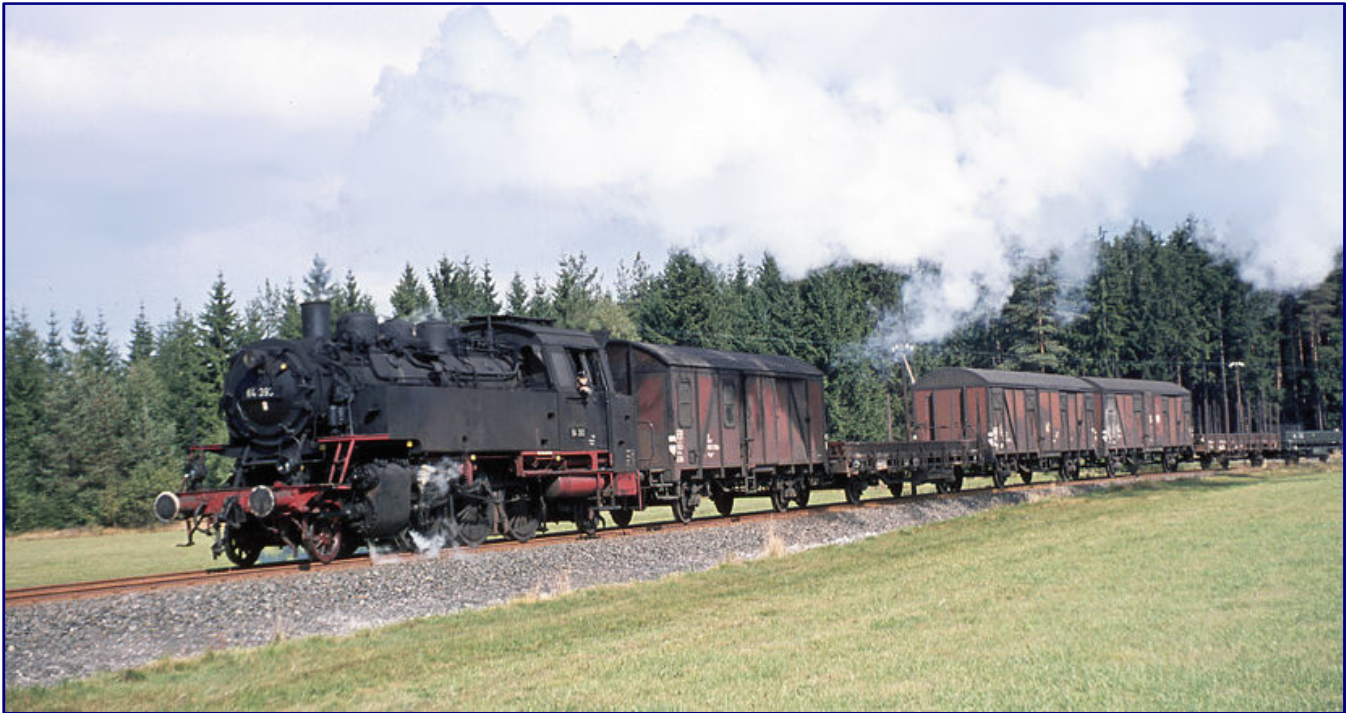
Also in the short short-distance freight train 16185 to Eslarn, led by 064 393-2, two covered wagons Gbs according to the UIC standard were listed on September 12, 1973. Photo: Peter Schiffer / Eisenbahnstiftung
