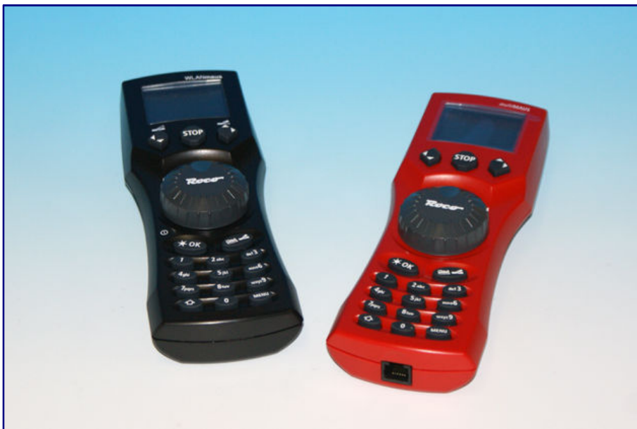
The multi-central unit from Roco (right), which is also used in Z gauge, is both a handset control and a small central unit. It can also switch points or mechanical signals. Its modern successor is the WLAN mouse (left) from the same manufacturer.
