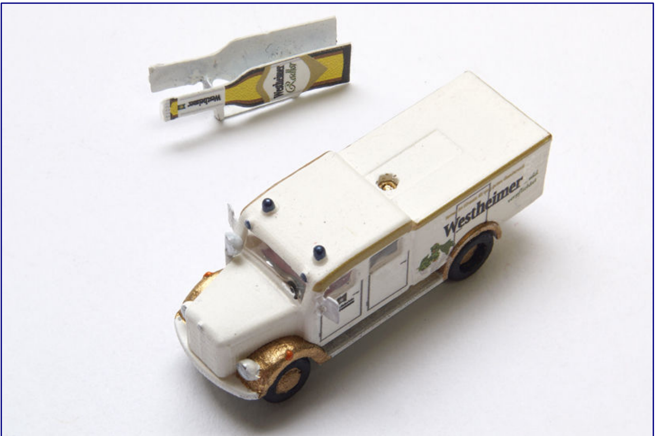
On the Westheimer vehicle, too, all three vehicle parts and the roof plate are ready (photo above). They are connected with a micro-screw that is guided through the chassis from below and engages in the nut resting in the body (photo below).
