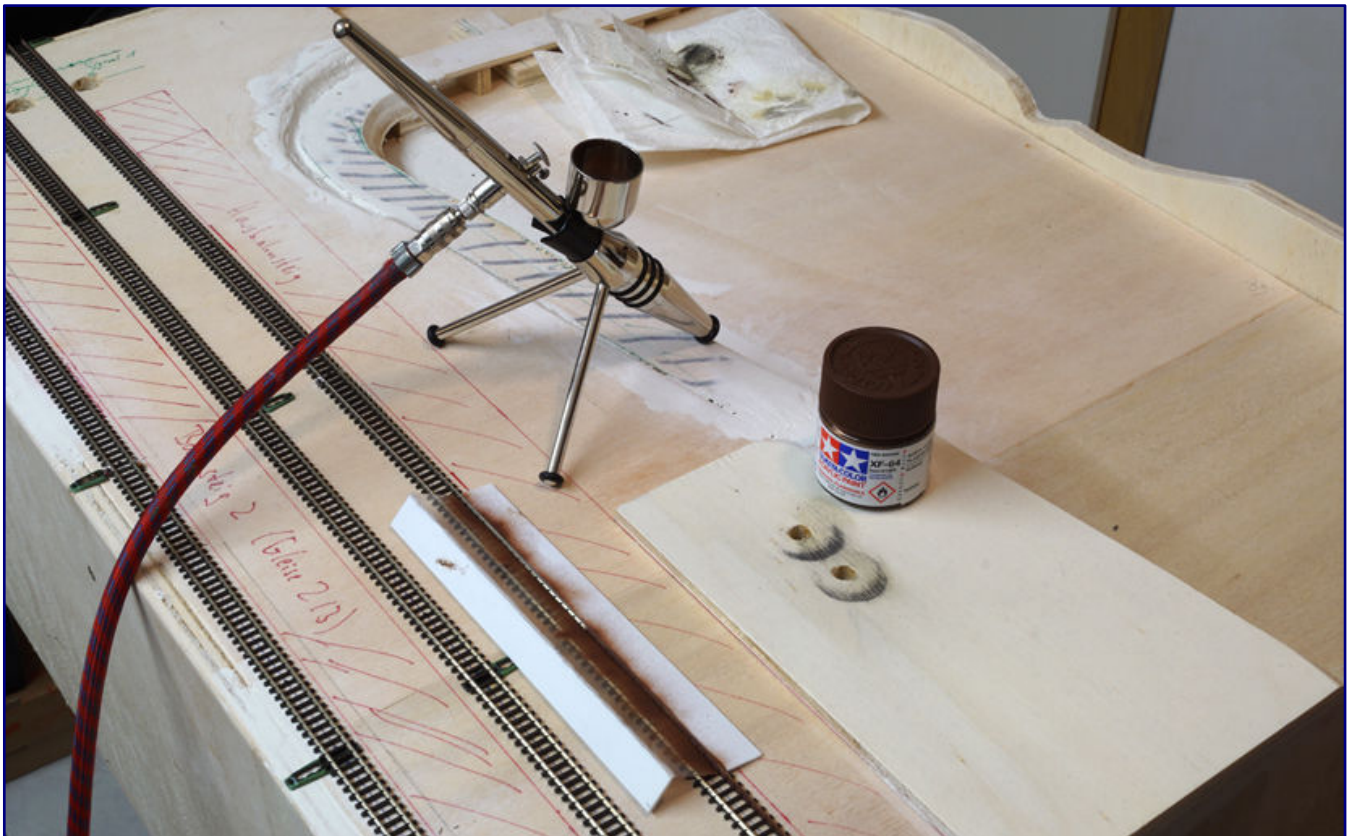
The rail flanks get a rust patina with air-brushed Tamiya paint. In order to keep paint from unwanted areas, we use a self-made spray stencil made of polystyrene pieces.
