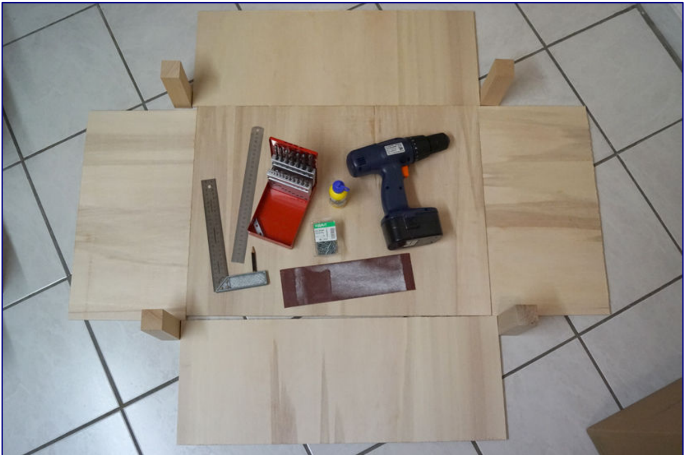
Before the wooden box is assembled, all parts are laid out once again for checking their correct fit.
