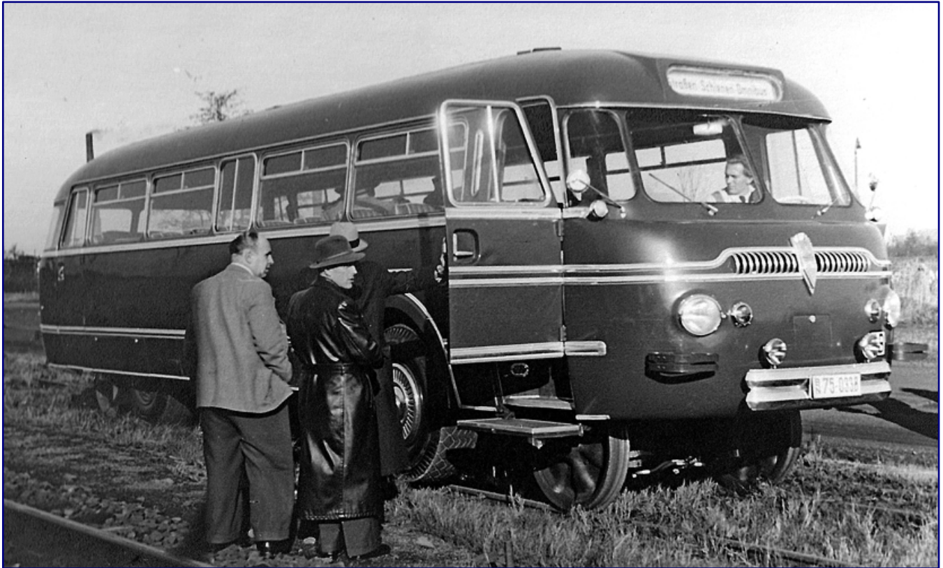
A historical document of inestimable value today has been slumbering in the family album for decades: It shows the prototype V4, ancestor of all modern rail-road vehicles, during its acceptance by the German Federal Railroad in early 1954. The registration number shows that the vehicle was converted for this unique piece, which can also be seen on pages 20 and 23. Photo: Archive Kaiser
