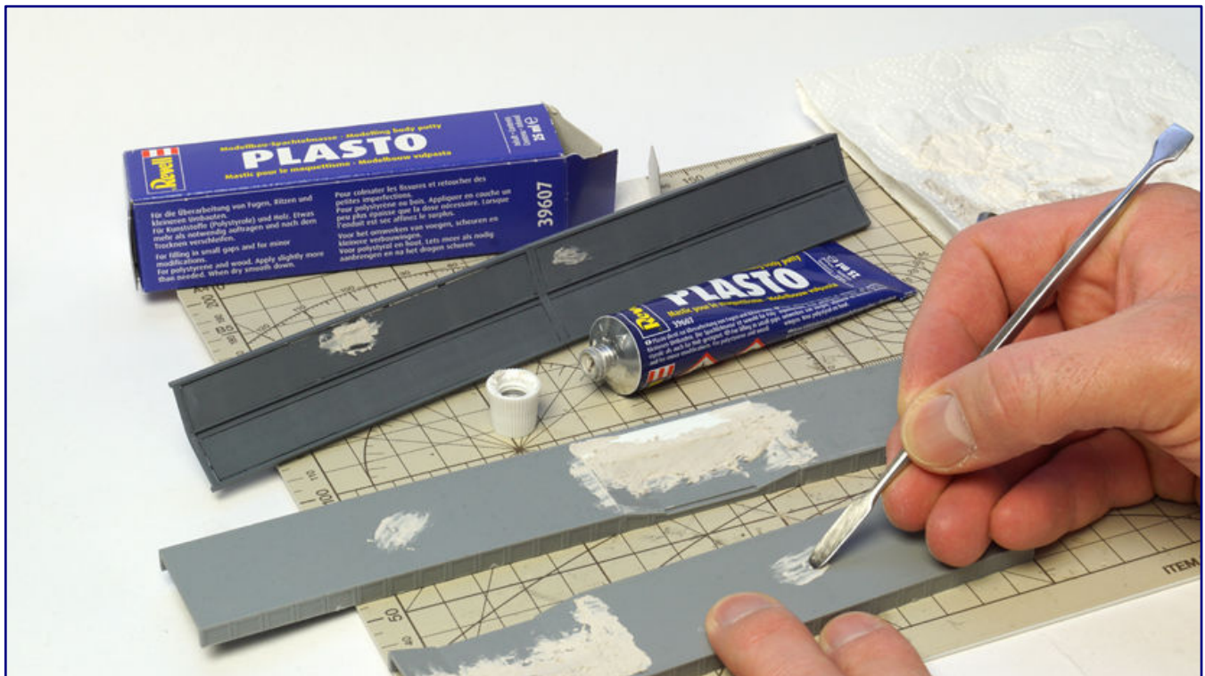
The kit-bashed parts are filled and sanded before being painted.
