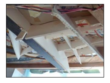
The terrain between the upper table-top, which carries the tracks and the station area, and lower edge of the layout is made up of interlaced foamboard formers clad as per the text.
