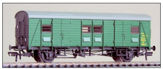
**Model Details:** The model illustrated is in BR Southern Region coach green livery (era 5) as number S1511S. This indicates that it started life on the Southern Railway and the absence of end doors makes it a PLV. It needs to be handled with care as the fine detail below floor level can easily be damaged. It has fine wire grab rails on each corner and comes with brake hoses and dummy coupling hooks ready fitted. The recommended retail price is £29.95.
